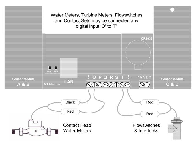
**Typical Sensor Driver Connections**
