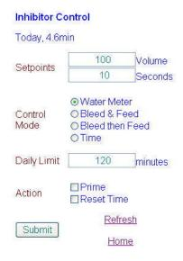
Conductivity-Bleed, Inhibitor, pH-Acid & Biocide Controls Controller Type: CO-IN-PH-TB with option LB
