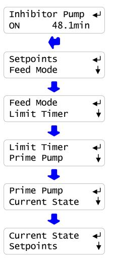
Sidebar: Prime Pump will not turn ON the Pump if the flowswitch is OFF.
