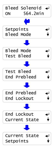
Sidebar: Test Bleed will not turn ON the solenoid if the flowswitch is OFF.
