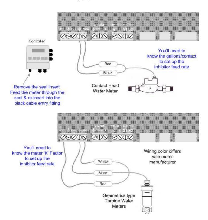
Do not install meter cabling in the same conduit at AC power wiring.
