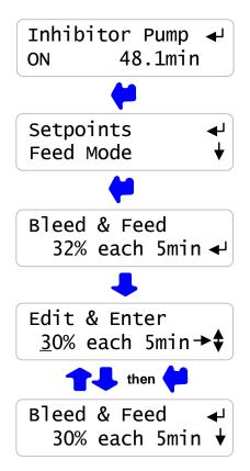
**Sidebar:** Bleed & Feed is the most common but usually not the best way to feed inhibitor.
