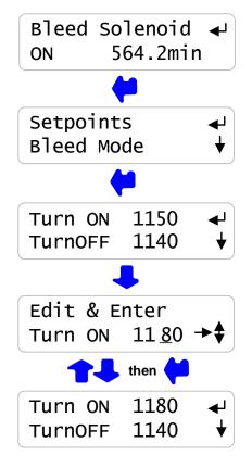
**Sidebar:** The difference between Turn ON & TurnOFF, the 'deadband', is usually set to 10uS. If you are watching the tower conductivity as the sump float turns the make-up water ON & OFF, you'll observe the operational deadband exceeds 10uS.
