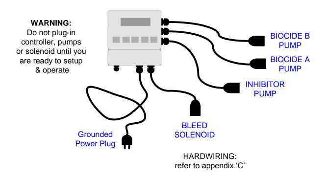
You may be using a pot feeder controlled by a solenoid to an oxidant as either Biocide A or B. Verify that it's plugged into the middle or lowest of the three enclosure sidewall sockets.
