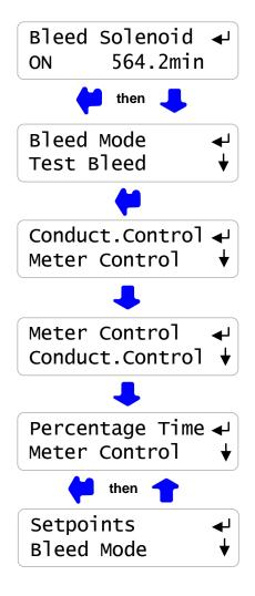
**Sidebar:** 'Meter Control' mode is used where sensor fouling from silica or organics continuously fouls the conductivity sensor.
