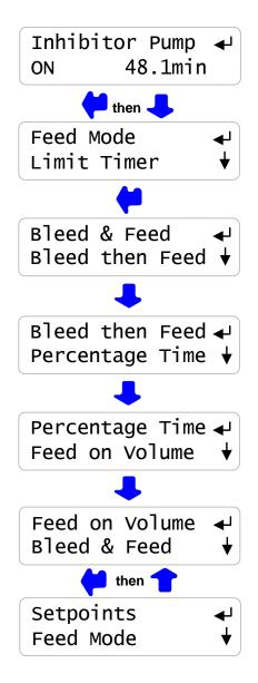
**Sidebar:** Bleed & Feed is used on bleed limited towers where the bleed solenoid is ON for more than 50% of the time.
