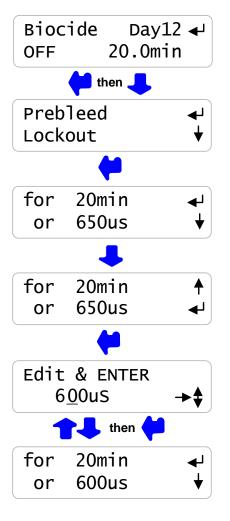
**Sidebar:** Prebleeding turns on the bleed solenoid before each biocide event to lower the tower conductivity. Prebleeding limits bleed and sewering of the biocide during the 'kill time'
