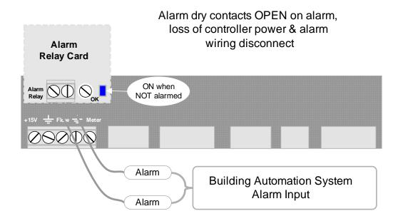
Wire alarm contacts AWG22 to AWG18, 2 conductor
