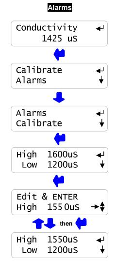
**Sidebar:** Conductivity alarms may occur when the tower shuts down and drains the sample line or when a Biocide event Prebleed, lowers the conductivity.
