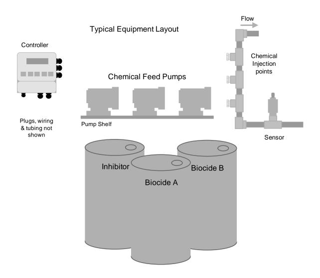
Although sensor cables and pump tubing may be extended, ease of servicing occurs when water treatment components are located in the same area.
