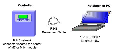
Controllers use a static IP address to communicate using TCP/IP 10 base T. Site IT provides LAN IP addresses and they may also wish to modify the ports used for HTML (default 80) and Telnet (default 23). They may also require the controller MAC.
