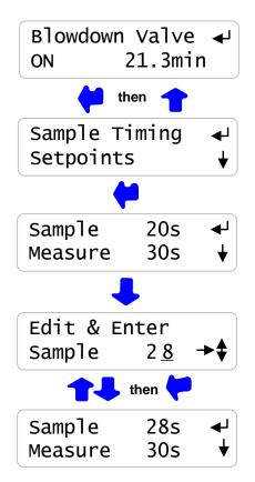
**Sample:** May be set a short as 5 seconds if the sensor is located at the boiler or as long as 60 seconds for a sensor 100 feet from a boiler. It's the time required to fill the piping between boiler & sensor and reflects both the length of pipe and the setting of the throttling valve.
