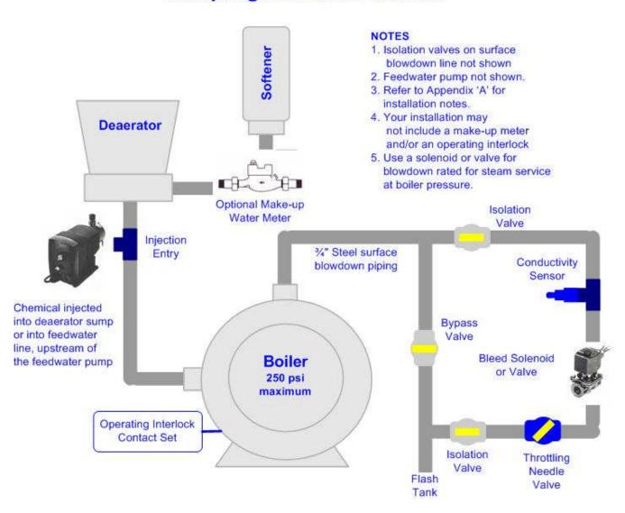
Sampling Blowdown Control is the most commonly used blowdown method. It provides the most accurate control at the lowest energy and chemical cost for most boilers and it's relatively insensitive to the setting of the throttling needle valve.
