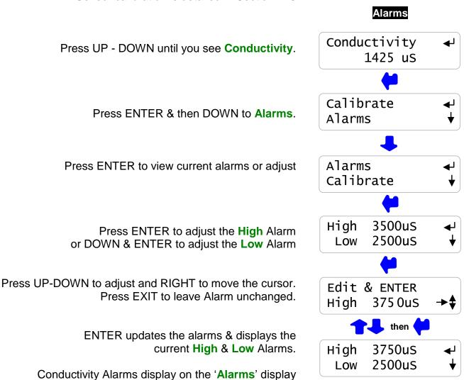
'Clear Alarms' does not reset a conductivity alarm above the High or less than the Low Alarm level.
