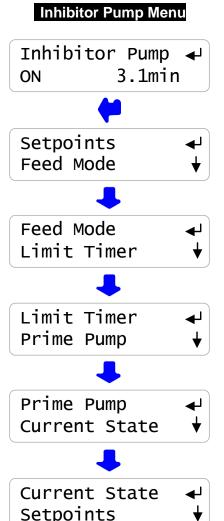
Sidebar: Prime Pump will not turn ON the pump unless Interlock is ON.
