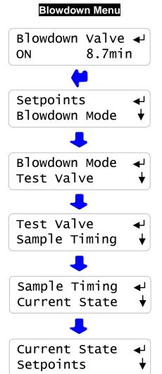
Sidebar: Test Blowdown will not turn ON the Blowdown Valve unless the Interlock is ON.
