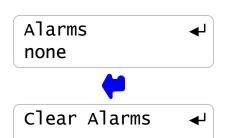
Press ENTER to **Clear Alarms**. Clearing alarms sets pump & blowdown owed times to zero.
