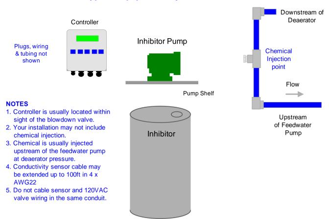
Although sensor cables and pump tubing may be extended, ease of servicing occurs when water treatment components are located in the same area.
