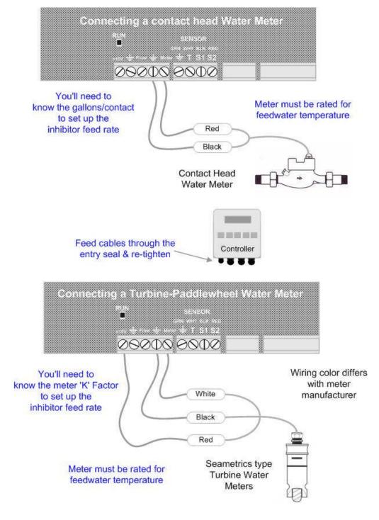
Do not install meter cabling in the same conduit as AC power wiring.
