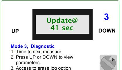
**Update**@ counts down to next corrosion rate measurement.
