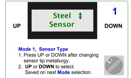
The LogR is set for the tip metallurgy ordered with the LogR. If you change the tip metallurgy, use Mode 1 to select the tip metal or alloy.
